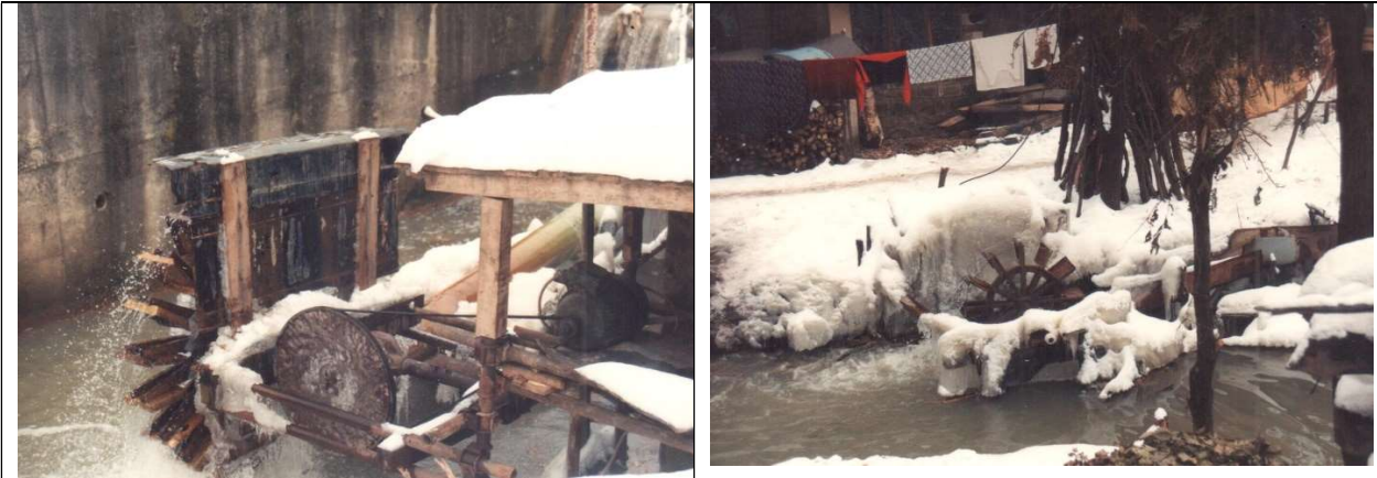
Above: Since the supply of electrical power had been cut off as part of the siege, some of the local workmen had built their own hydro-electric power generating stations.
